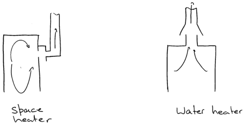
Figure A Typical draught diverter and flue arrangements: Purpose is to secure flame stability
